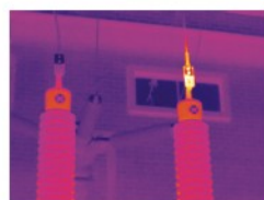
Sleeve connection overheating
