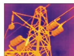
High voltage wire porcelain set overheating
